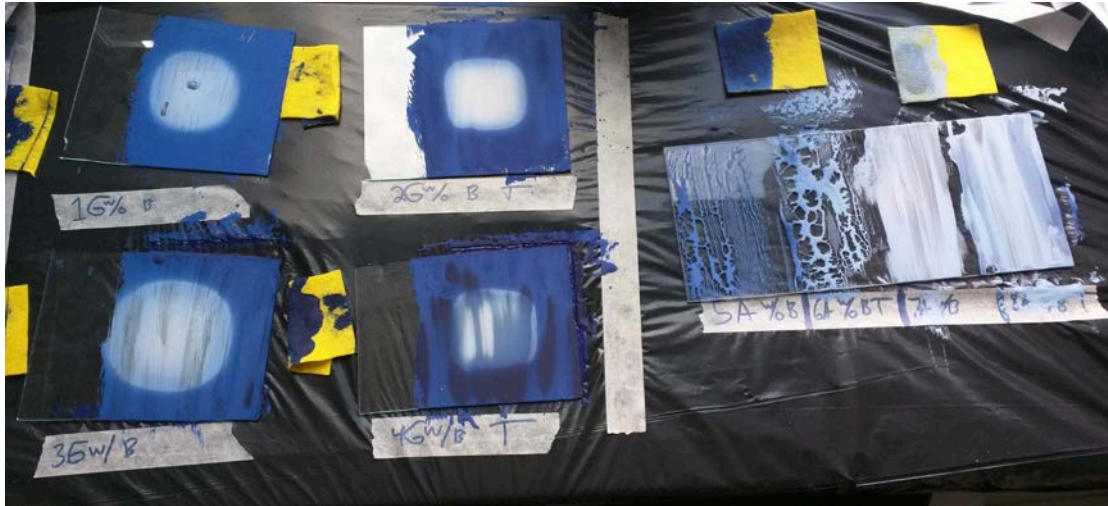
Figure 25: Semi-Failed experiments with making thermochromic paint.
